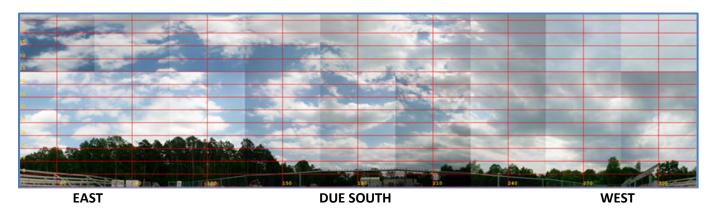
The ASSET software projects the path of the sun throughout the year and calculates the shading factor as **96.8%**, adjusted for deciduous trees. Thus on an annual basis, the array will experience **3.2%** energy production losses due to shading, on average. The simple average of monthly shading is 3.5%, but the highest shading losses occur during low energy production months.
